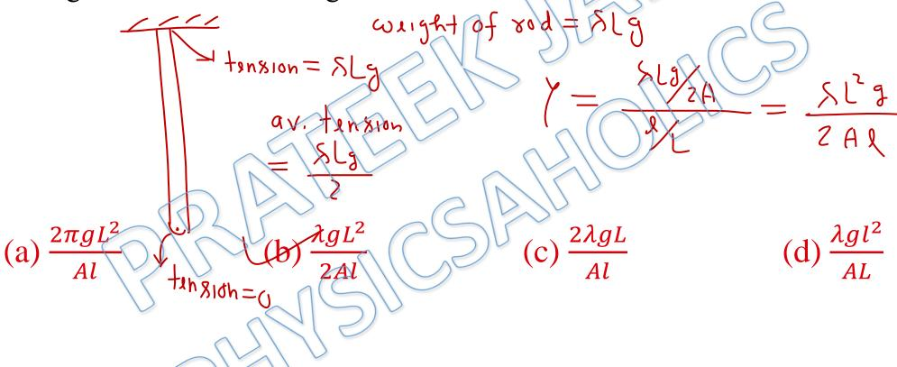
Q6) A uniform slender rod of length L, cross-sectional area A and Young's modulus Y is acted upon by the forces shown in the figure. The elongation of the rod is
